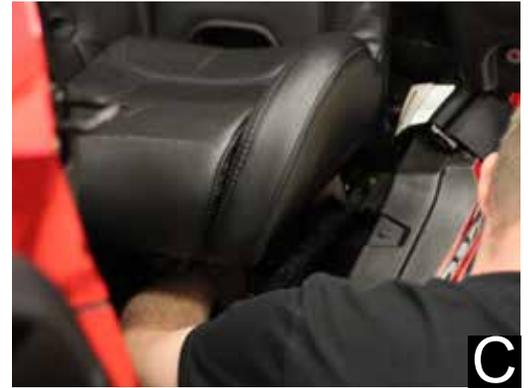
**Step 6:** You can now put your driver side seat in the car, tighten the 4 hex nuts. In order to reach the rear nuts you will have to reach under the seat with a socket wrench. **Figure-C**
